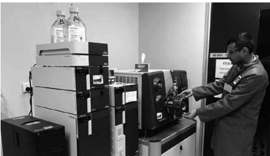
The mass spectrometer used to test wastewater
